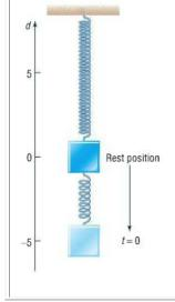
Suppose that the displacement d (in meters) of an object at time t (in seconds) satisfies the equation  $d = 10 \sin(5t)$
